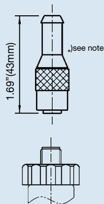
Flying leads conductor cross section up to max. 0.5 mm<sup>2</sup> / AWG 20 with end splices, conductor outer diameter 6.8 mm, NEMA 4 / IP 67
