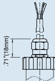
Cable with free ends, adjustable zero and span conductor cross section up to max. 0.5 mm<sup>2</sup> / AWG 20 with end splices, conductor outer diameter 6.8 mm, NEMA 6 P / IP 68
