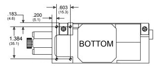
ALL DIMENSIONS UNLESS OTHERWISE SPECIFIED .XXX ±.008 (.02mm) (MILLIMETERS SHOWN IN BRACKETS)
