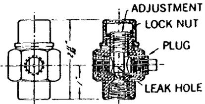
All parts made of brass, 1/4" pipe connections. Pipe plug may be removed for installation of pressure gauge. No. 94204-A2 is available without leak hole.
