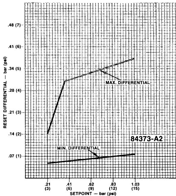
**Reset Differential Range:** See graph corresponding to instrument model numbers.
