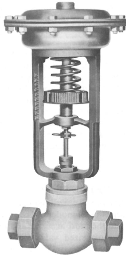
The setpoint is changed by varying the load on the adjusting spring. Rotating the ball-bearing adjustment wheel so as to compress the spring and increase its force against the diaphragm raises the setpoint. Rotation in the opposite direction lowers the setpoint. The scale along one side of the frame provides a reference for restoring the setpoint when adjustment wheel position has been changed from its normal setting.
