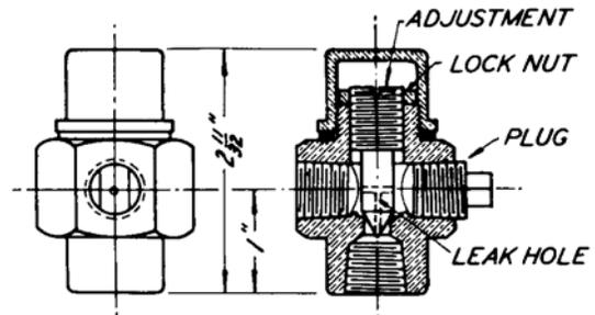
Most types of pressure regulators require a "feeler" pipe for best control. By using this adjustable orifice in the feeler pipe line, rapid pressure fluctuations will be dampened out and more steady control procured.
