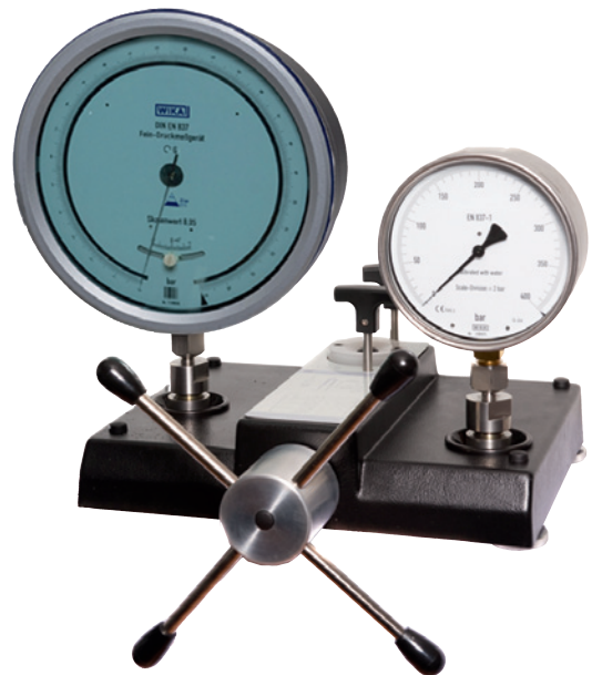
Calibration assembly CPP1200-X with test gauge as reference instrument and test item
