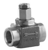
Chemiquip recommends the use a chemiquip snubber with the limiting valve. The snubber is attached to the inlet port and its function is to (1) dampen any pressure pulsations before they reach the valve and gauge and thereby assure a smooth response and accuracy of the valve to pressure changes and (2) prevent the entrance of any solid contamination into the valve.
