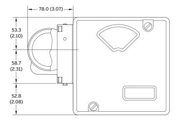
Figure 7 View with explosion proof I/P converter
