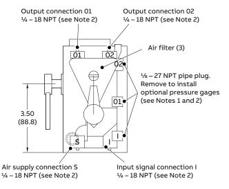
Figure 9 View with optional manifold
