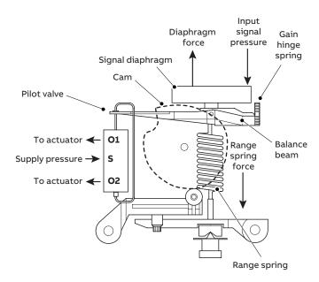
Figure 3 Operation diagram
