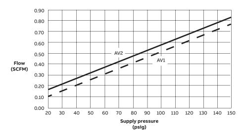
Figure 1 Air consumption (at null)
