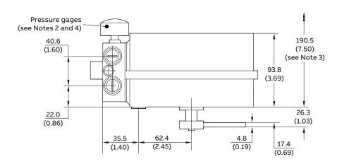
Figure 6 External and mounting dimensions (shown with optional bypass manifold)
