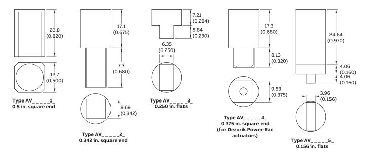
Figure 12 Drive shaft options dimensions
