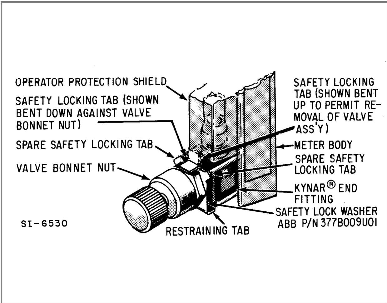
**FIGURE 4-1. VALVE STEM ASSEMBLY FOR KYNAR END FITTING**
