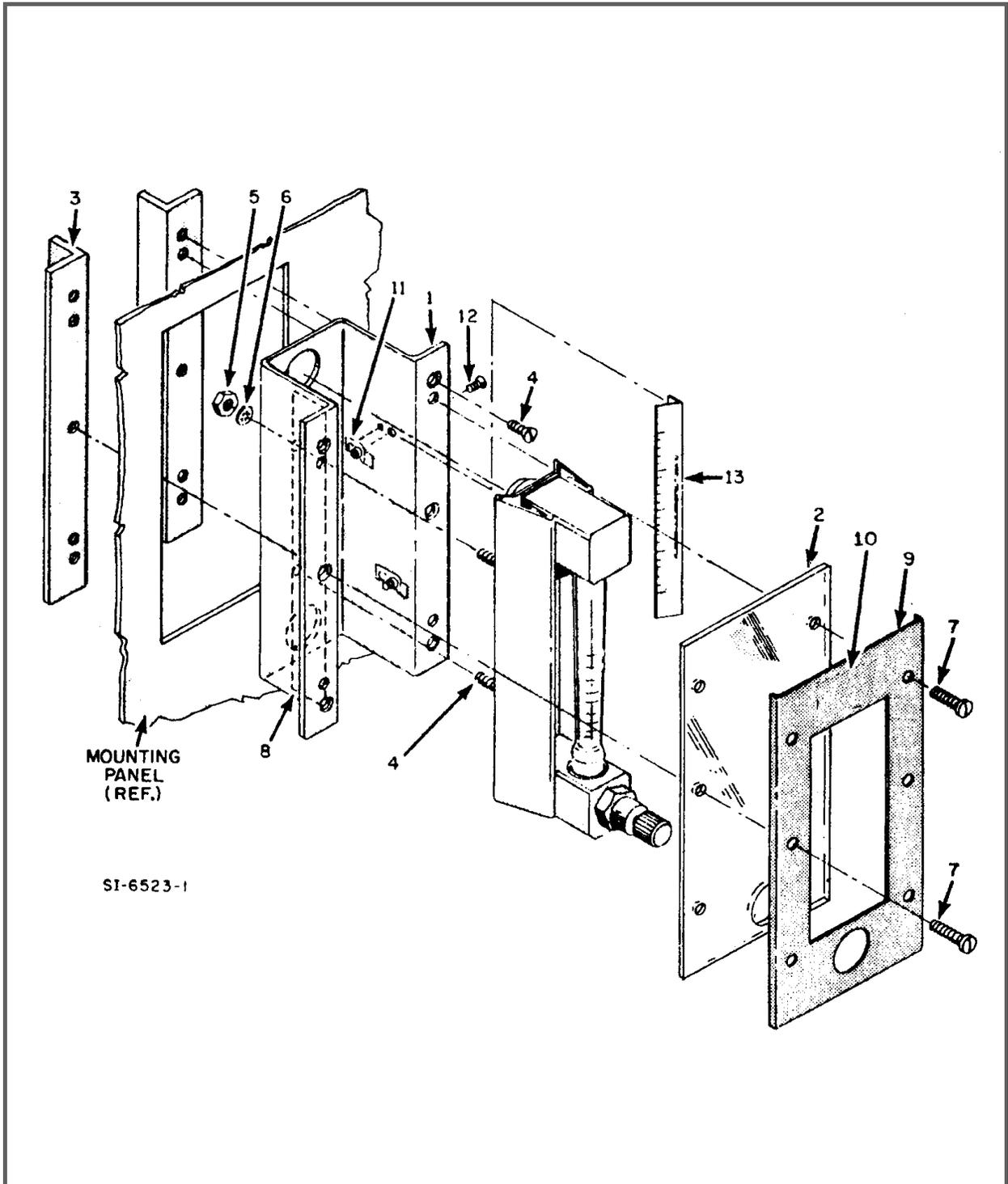
FIGURE 5-5. MODEL 10A6130 FLUSH PANEL MOUNT PARTS
