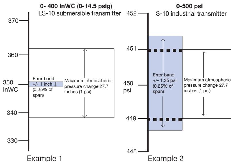
Industrial transmitters less than 400 psi span must be vented, since atmospheric pressure changes can be greater than the error band produced by the transmitter accuracy. *All WIKA Tronic piezoresistive transmitters with gauge, compound, or vacuum pressure ranges are vented to atmosphere.*
