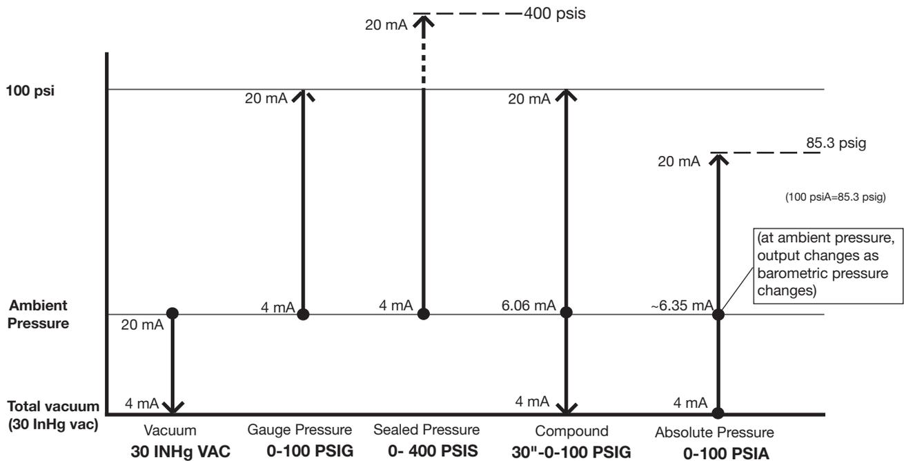
For transmitters with standard output signals, the rule "*the higher the pressure, the higher the output signal*" applies for all pressure references, compound, and vacuum ranges. Transmitters with reverse output (such as 20-4 mA) are available for special requirements.
