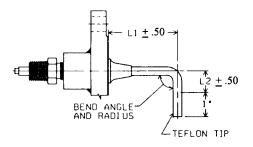
For insulated sheath option, sheath must terminate 2" or more before start of bend.
