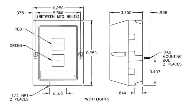
Mounting Dimensions for Model 310 Level-Tek with Explosion Proof Display Unit
