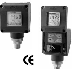
The UniTrans pressure transmitter is designed for a variety of pressure measurement applications. Durable construction includes all stainless steel wetted parts for compatibility with a variety of media. The Type UT-10 is supplied with a 1/2" male NPT process connection. The Type UT-11 features a flat, non-clogging flush diaphragm process connection for use with highly viscous or crystallizing media, or media containing solids.
