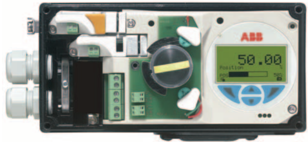
Fig. 6: Open positioner with view of LCD indicator
