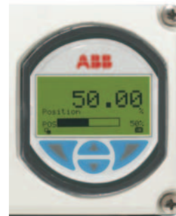
Fig. 7: LCD indicator with pushbuttons and LCD display
