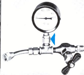
Kent-Moore power steering tester. Snubber damps pump pulsations.
